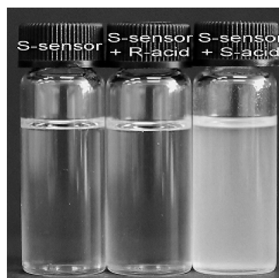
FIGURE 10. Images of ( S )- 14 ( 5.0 \times 10^{-4} M in benzene/0.4% v DME) with ( R )- and ( S )-MA ( 4.0 \times 10^{-3} M).
